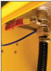
Suction pipe with inlet filter and drain hose is located in wash pail.
