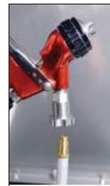
Placing Spray Gun on Nozzle Extension
