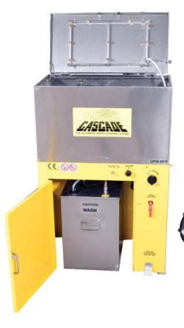
SOLVENT FLOWS FROM OVER 40 JETS IN THE CLEANING TANK TO WASH DEBRIS FROM INDUSTRIAL PARTS.
