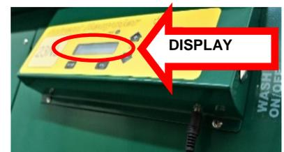
Upon the temperature of Boiler Tank dropping down to the pre-set value, LCD shows READY status. Residue Drain Valve located at the bottom of the Boiler Tank may be opened to drain all oily residues into Residue Drawer as shown in the photo.
