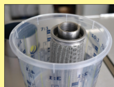
Clean Metal Filter in Solvent
