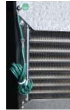
Ground wire located on back of recycler.
