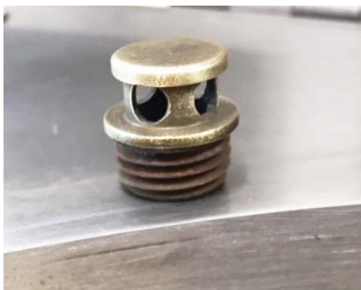
Figure 14. Vapour outlet fitting
