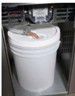
Figure 9. Place the HDPE receiving pail in the cabinet. Remove the cap. Position the discharge tube in the 3.0 cm opening.
