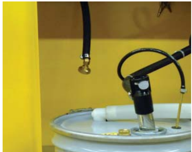
SOLVENT PAIL SETUP - METAL PAILS
