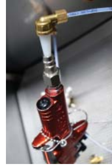
Air Plug inserted into the Air Passage way of the spray gun
