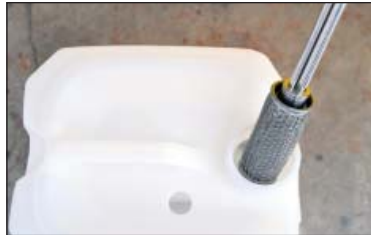
Remove Suction Pipe and Filter
