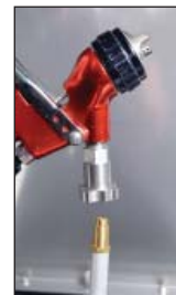
Placing Spray Gun on Nozzle Extension
