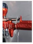
Trigger Lock Spring On Spray Gun
