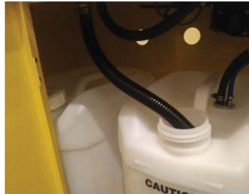
DRAIN HOSE MOVED TO CLEAN (RIGHT) PAIL TO FILL CLEAN PAIL
