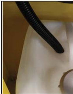
DRAIN HOSE IN WASH (LEFT) PAIL
