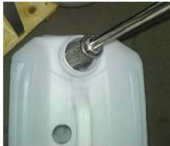
B, Remove Suction Pipe and Filter
